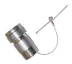
The Sigma 316 stainless steel, pressure relieving Fill Cap prevents pressure accumulation within a Hydraulic Reservoir (Storage Tank). It will exhaust the gas before accumulation can occur, through the spring-loaded cover assembly.
