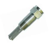
The Sigma 316 stainless steel, pressure relieving Fill Cap prevents pressure accumulation, within a Hydraulic Reservoir (Storage Tank). It will exhaust the gas before pressure accumulation can occur, through the spring loaded cover assembly.
