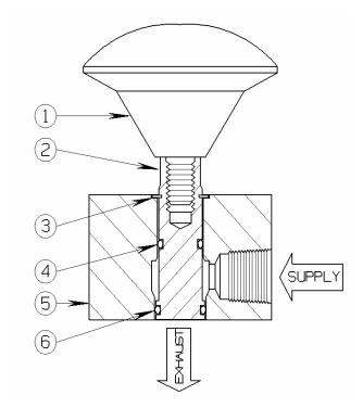
The **16RS18** is a two position, two-way normally\_closed, high flow capacity manually operated ESD control valve. In the shelf or normal placement, the valve has the Supply port blocked or isolated from the Exhaust port. Pulling outward on the ESD Valve's handle will establish a Supply-to-Exhaust flow path, rapidly depressurizing the ESD control circuit.
