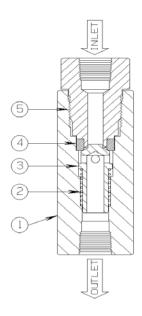
The **14KS Check Valve** is a two position, spring biased poppet operated flow control device that permits Inlet to Outlet flow only. Our Check or Flow Safety Valve (FSV) prevents reverse pressure flow from Outlet to Inlet through spring assisted poppet positioning.
