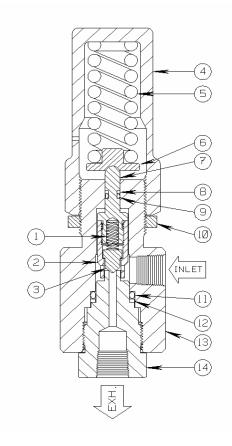
The **24RV14** is a two position, two-way normally closed, pressure relieving (spring/sensing plunger operated), flow control valve. It has excellent pressure relief and reset repeatability. Relief Valves or Pressure Safety Valves (PSV) are most commonly used to prevent abnormal pressure increases in hydraulic control circuits. As the operating pressure within a control circuit increases to or above a predetermined pressure setting, it will be dispersed through the Relief Valve's Exhaust port.
