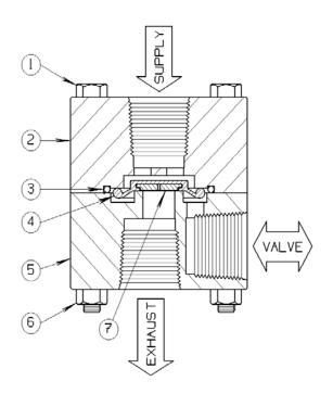
The **13QS42/43** is a two position, Flapper Seal operated, control valve assembly with <a href="https://high.nlm.nih.google.com/high.flow/exhaust">high flow/exhaust</a> capacity. This 1/2-14 N.P.T. valve has a maximum operating pressure of 150 PSI. It establishes flow from the Supply to Valve connections (inlet to outlet) to open a Surface Safety Valve (SSV or pneumatic Actuator), automatically with each application of operating pressure.
