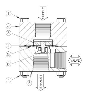
The **13QS27** is a two position, Flapper Seal operated, <u>high</u> <u>flow exhaust</u>, control valve assembly. It establishes flow (from the inlet to outlet or Supply-to-Valve connections) to open a Surface Safety Valve (SSV or pneumatic Actuator), automatically with each application of operating pressure.
