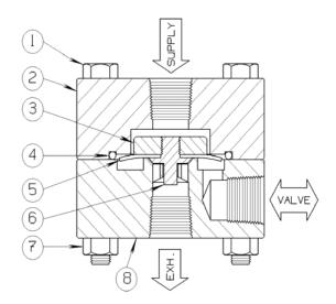
The **13QS23** is a two position, Flapper Seal operated, <u>high</u> <u>flow exhaust</u>, control valve assembly. It establishes flow (from the inlet to outlet or Supply-to-Valve connections) to open a Surface Safety Valve (SSV or pneumatic Actuator), automatically with each application of operating pressure.
