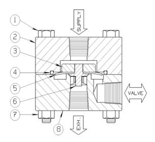
The **13QS15** is a two position, Flapper Seal operated, <u>high</u> <u>flow exhaust</u>, control valve assembly. It establishes flow (from the inlet to outlet or Supply-to-Valve connections) to open a Surface Safety Valve (SSV or pneumatic Actuator), automatically with each application of operating pressure.
