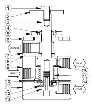
The **11RRS93-94** is a two position, three-way normally closed block and bleed Manual Reset Relay valve. It is designed to establish Supply-to-Valve output pressure (generally 50-150 PSI) with a manual **Pull** of the valve handle. To close the valve, **Push** on the valve handle to release downstream pressure.
