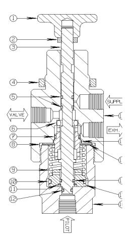
The 11LV36 is a two position, three-way normally closed block and bleed Manual Reset Relay valve. It is designed to establish Supply-to-Valve output pressure with manual **Pull** positioning of the Knob.
