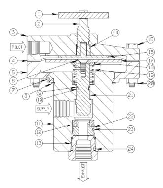
The **20HM20** is a two position, two-way normally open, Pilot Supply pressure operated, **high flow** control valve assembly. It is designed to block incoming hydraulic Supply pressure automatically when relatively low Pilot Supply pressure is applied.
