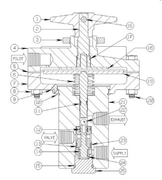
The **20HM104** is a two position, three-way normally closed, Pilot operated, hydraulic flow control valve assembly. It is designed to establish high-pressure hydraulic fluid output, automatically with each application of Pilot Supply pressure.
