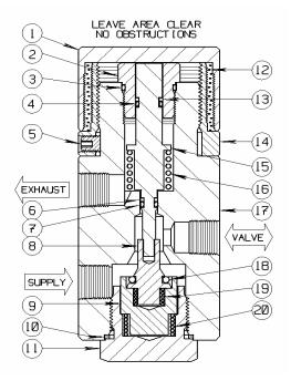
The 15RS84 Fusible Valve is a two position, three-way normally open Block & Bleed, <u>Temperature Sensitive</u> flow control device. When intense heat or close proximity to a fire causes the valve temperature to exceed the eutectic melting point, valve springs (Items 16, 19 and 20) decompress moving Poppet (Item 8) to block inlet supply pressure and vent downstream (receiving circuit) pressure out the Exhaust port.
