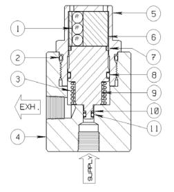
The 15RS66 Fusible Valve is a two position, two- way normally closed, **Temperature Sensitive** flow control device. Intense heat, or close proximity to a fire, will melt the solid Eutectic that maintains the valve's normally closed flow path. When the valve is subjected to heat that exceeds the actuation temperature, a Supply-to-Exhaust flow path will occur automatically.
