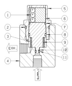
The 15RS57 Fusible Valve is a two position, two-way normally closed, <u>Temperature Sensitive</u> flow control device. Intense heat, or close proximity to a fire, will melt the solid Eutectic that maintains the valve's normally closed flow path. When the valve is subjected to heat that exceeds the actuation temperature, a Supply-to-Exhaust flow path will occur automatically.
