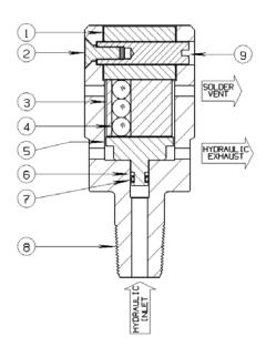
Sigma 2-Way Fusible Valves are two position, two- way normally closed, <u>Temperature Sensitive</u> flow control device. Intense heat or close proximity to a fire will melt the solid Eutectic that maintains the valve's normally closed flow path. When the valve is subjected to heat that exceeds the actuation temperature, a Supply-to-Exhaust flow path will occur automatically.
