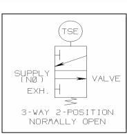
The 15RS128/129/164 Fusible Valve is a two position, threeway normally open Block & Bleed, <u>Temperature Sensitive</u> flow control device. When intense heat or close proximity to a fire causes the valve temperature to exceed the eutectic melting point, valve springs (Items 5, 6, and 16) decompress moving Poppet (Item 15) to block inlet supply pressure and vent downstream (receiving circuit) pressure out the Exhaust port.
