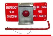
The **16RS48** is a glass enclosed, stainless steel, Emergency Shutdown (ESD) Station with easy-view large letters and a red background. It has a 1.00 Inch Diameter panel hole for installation of the 16RS36 (2W-N.C.) ESD valve. A striker is connected via stainless cable for breaking glass and accessing valve handle.
