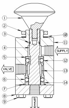
The **16RS40** is a two position, three-way normally\_open, high flow capacity manually operated block and bleed ESD control valve. In the normal placement (handle pushed in), the valve has a flow path established between its ports labeled Supply and Valve. Pulling outward on the handle will block incoming supply pressure and establish a Valve-to-Exhaust flow path, rapidly depressurizing the ESD control circuit.
