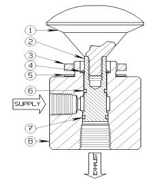
The **16RS36** is a two position, two-way normally closed, high flow capacity manually operated ESD control valve. In the shelf or normal placement, the valve has the Supply port blocked or isolated from the Exhaust port. Pulling outward on the ESD Valve's knob will establish a Supply-to-Exhaust flow path, rapidly depressurizing the ESD control circuit.
